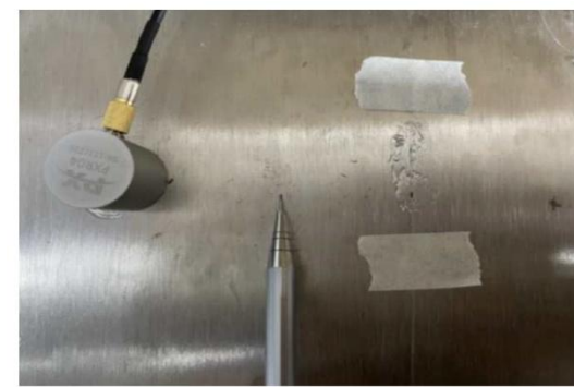
Acoustic emission sensor installed on a turbine blade
