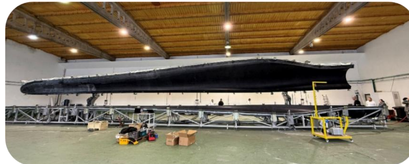
3D CAD geometry and one of Norvento's wind turbine blade moulds.
